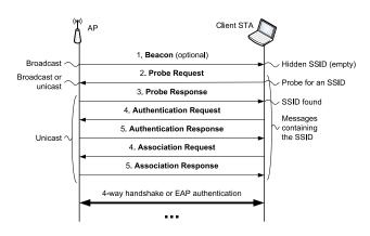
Figure 1: 802.11 network discovery and association with a hidden SSID or active probing (in active probing, the beacon is not sent)
